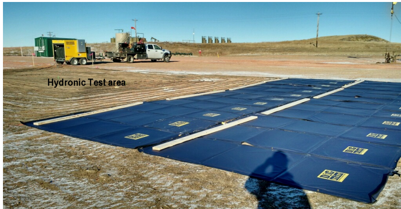
Above: DIG Ready Industrial Ground Thaw working against the Hydronic Test System (to left of DIG Ready mats)
